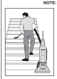
NOTE: Do not place the cleaner on furniture or steps for any period of time as the brush roll may cause damage. Place the cleaner on the floor with the handle in the upright/storage position while using the accessories. Do not allow the cleaner to tilt forward or to the side when using accessories. This will prevent the unit leaning ans causing possible damage to carpets or floors.
